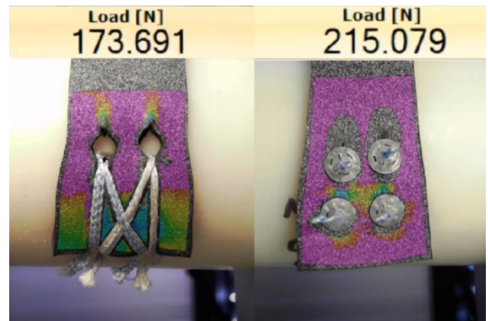
Double Row configuration (Flat Tape Like suture with 4 anchors) vs ZipE® Double Parallel construct (#2 suture with 2 anchors)
